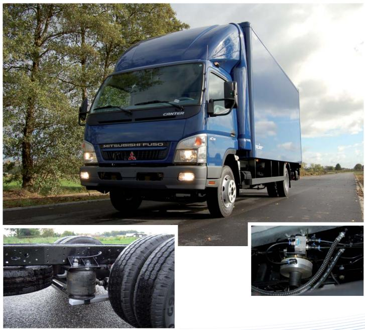
with VB-FullAir 2-Corner rear-axle air-suspension
